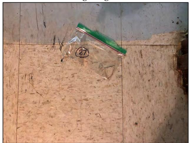
Sample #27 Asbestos containing floor mastic (under tile)
